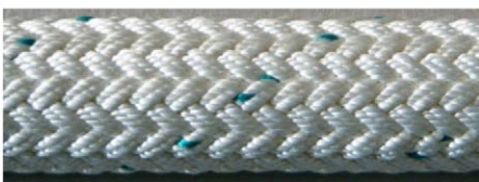
Figure 1 – Double-braided polyamide (PA) 100% rope
