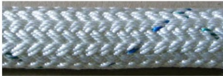
Figure 3 – Double-braided hibrid 1 (PA+ high elongation PET) rope
