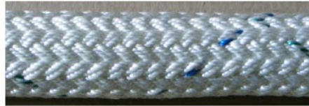
Figure 4 – Double-braided hibrid 2 (PA+ high tenacity with medium elongation PET) rope
